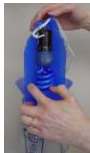
Light bulb should be flush against the vanes
