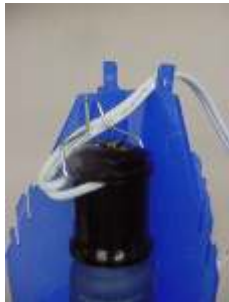
Hang the light unit in the hole towards the top of the vane as shown
