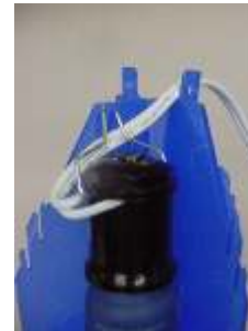
Hang the light unit in the hole towards the top of the vane as shown
